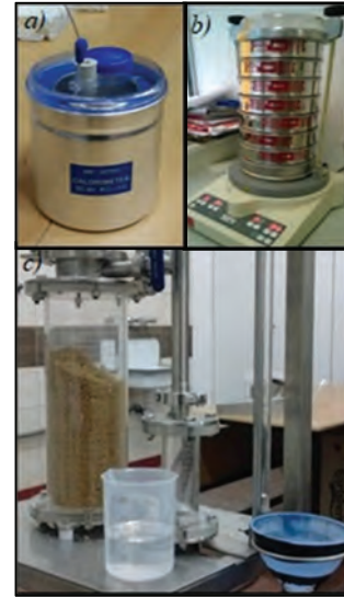
Figure 1: Measuring equipment: a) calorimeter, b) vibratory sieve shaker, and c) Hofsäss-type air pycnometer
