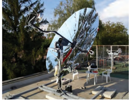
Fig. 1. The Physical model of the solar collector with spiral absorber
